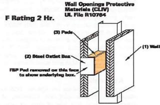
WALL ASSEMBLY - Constructed in the manner specified in the U400 series designs as shown in the UL Fire Registerica Directory.
